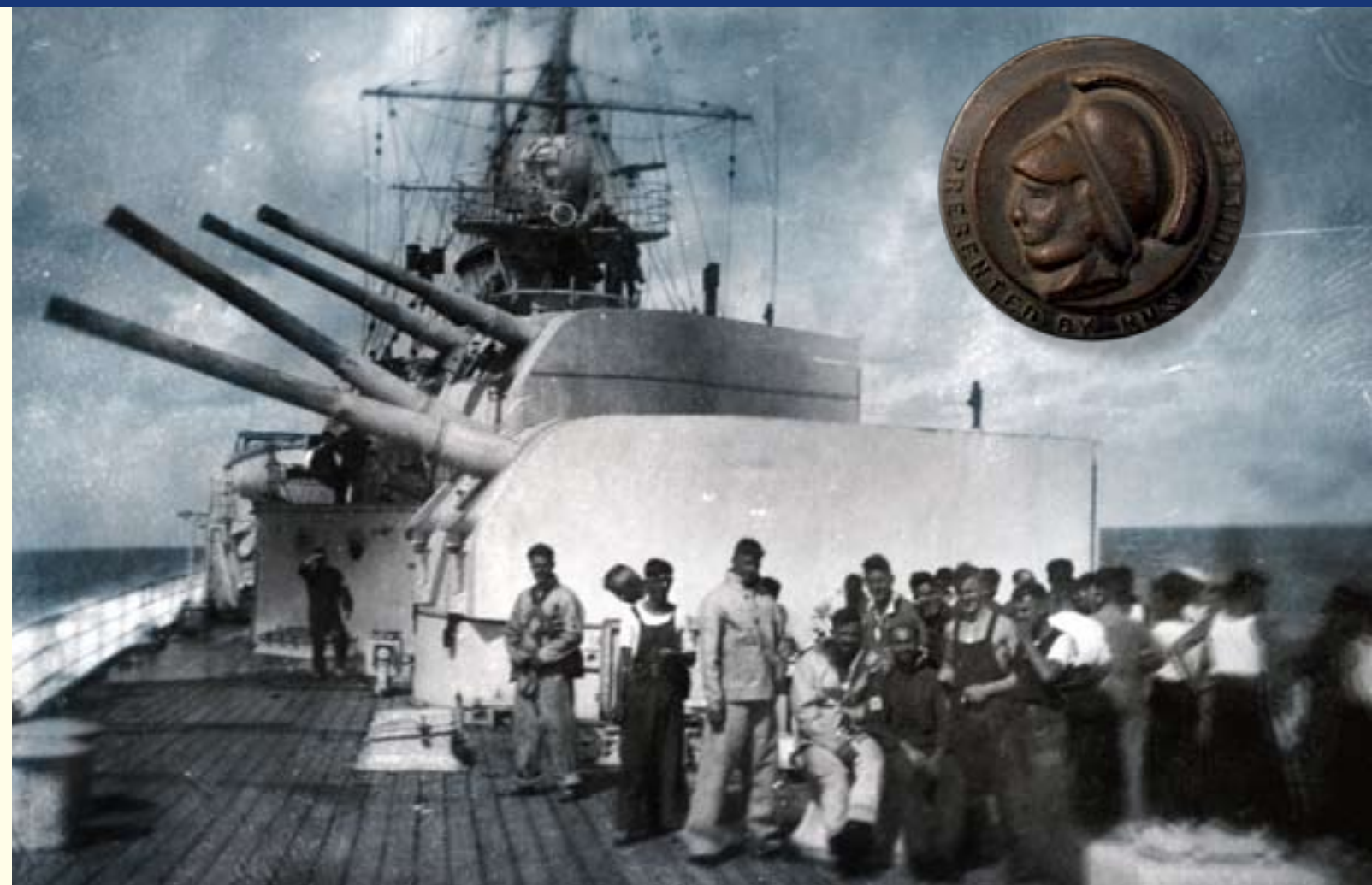
ABOVE: ACHILLES gun crews fall out on deck for fresh air, after the action. The turrets are still trained to port and the paint on the gun barrels has blistered from the heat of rapid firing.
