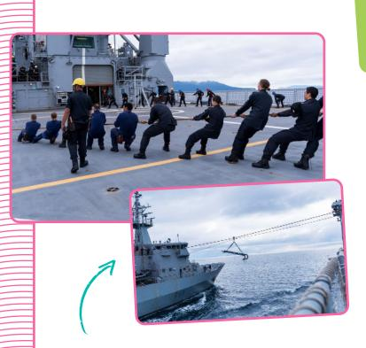
A jackstay passing a ladder between HMNZS Canterbury and HMNZS Wellington. The Navy personnel have to keep the line tight by hand!
